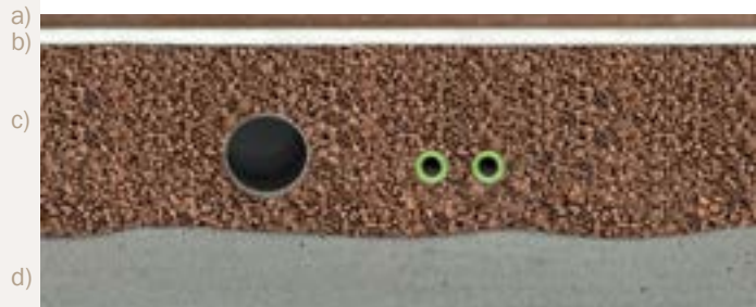
Solid ceiling with dry screed (floating)
