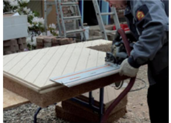
It can also be used for precise cutting by using the cutting stop.
