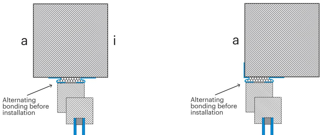
**Examples:** 2 prefabricated skirts on the window frame before window installation with double-sided Ampacoll® Fenax DS.
