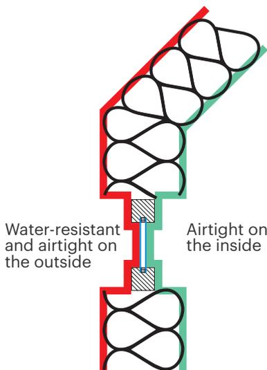
A building connection will retain its function in the long term if the layer on the inside and the windtight and driving rain impermeable layer on the outside are joined permanently and without gaps. This requires the creation of a sealing system with sufficient freedom of movement.
