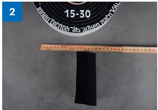
> Thickness of Ampacoll® Komprimax when not under tension.
