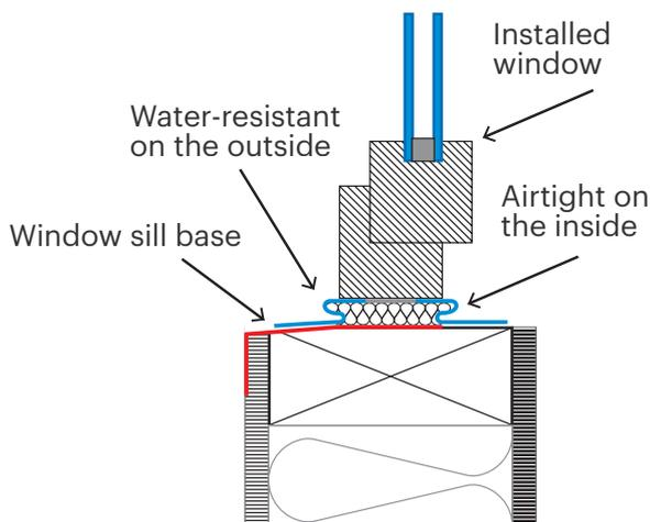
> If the windows are already installed in the factory, we recommend that the window sill base (as in solid construction) reaches at least up to the inner edge of the window frame. Of course, it can also cover the entire parapet depth.
