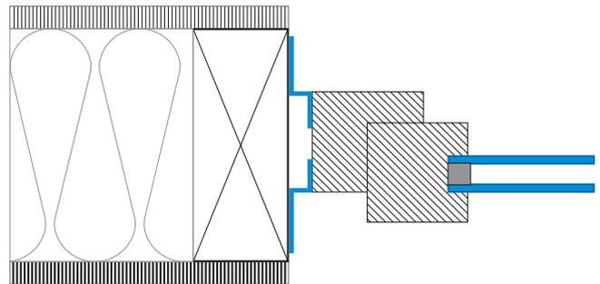
**Principle:** Both adhesive tapes before window installation. Alternating bonding.
