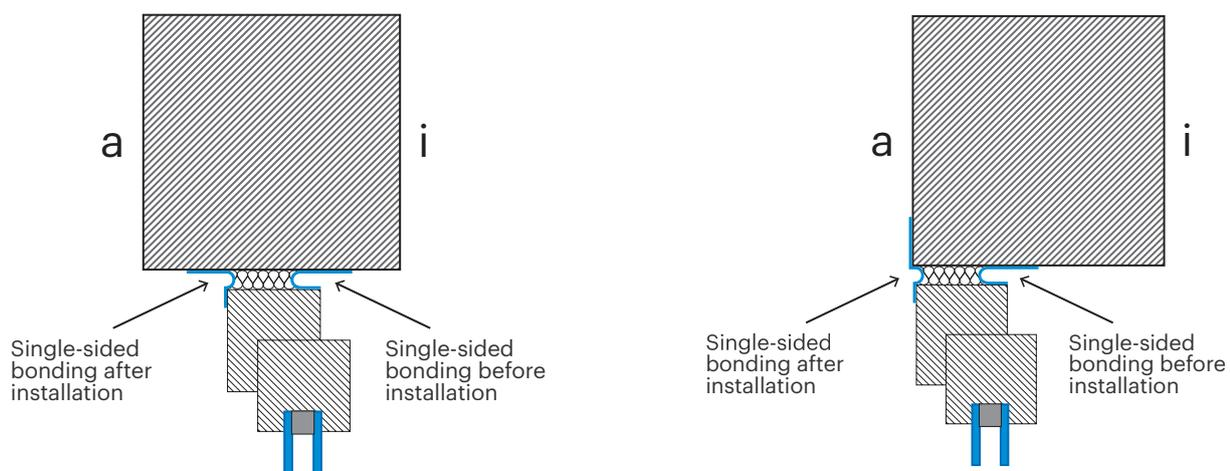
**Examples:** On the inside of the window (on the right in the picture), the tape was stuck to the window frame before the window was installed; on the outside (on the left in the picture), after the window was installed.
