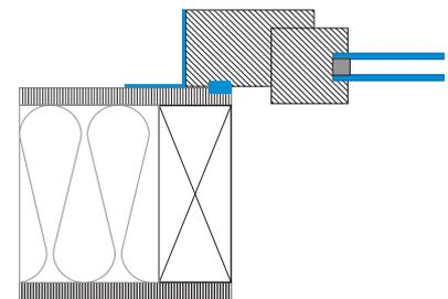
> Alternative with joint sealing tape or round cord
