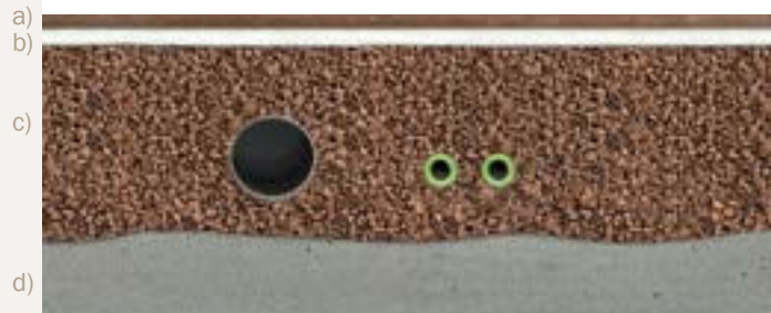
Solid ceiling with dry screed (floating)
