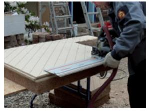
It can also be used for precise cutting by using the cutting stop.
