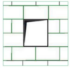
**ALTERNATIVE** Bond the tongue and groove connection around the whole circumference of the board using UdiSPECIAL ADHESIVE<sup>®</sup> Board offset  $\geq$  30 cm
