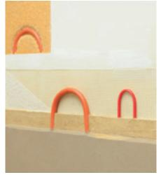
Wall heating systems can also be installed onto the plaster-finished surface. These should fixed securely to the substrate.
