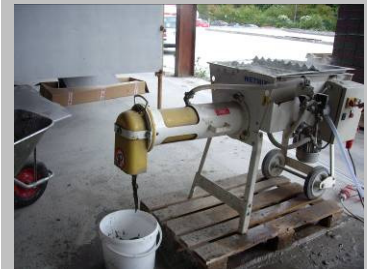
Fig. 2 Alternatively a horizontal mixer provides instantly mixed mortar at the touch of a button!
